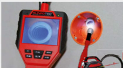
Pipe inspection from Ø 14 mm and more
